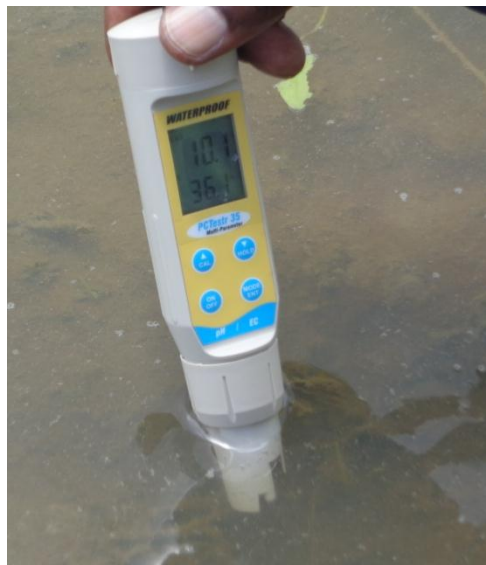
Plate 3.2 The PCTestr™ 35 Temperature/PH meter that was used to measure the dambo water pH and temperature. (Photo by Joel Lutomiah, 06.04.2013)
