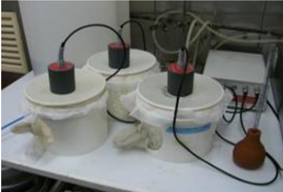
Plate 3.3: Mosquito feeding experimentation using Hemotek membrane feeder the feeder uses mice skin as a membrane to allow the mosquito obtain infectious blood meal from the mice skin.
