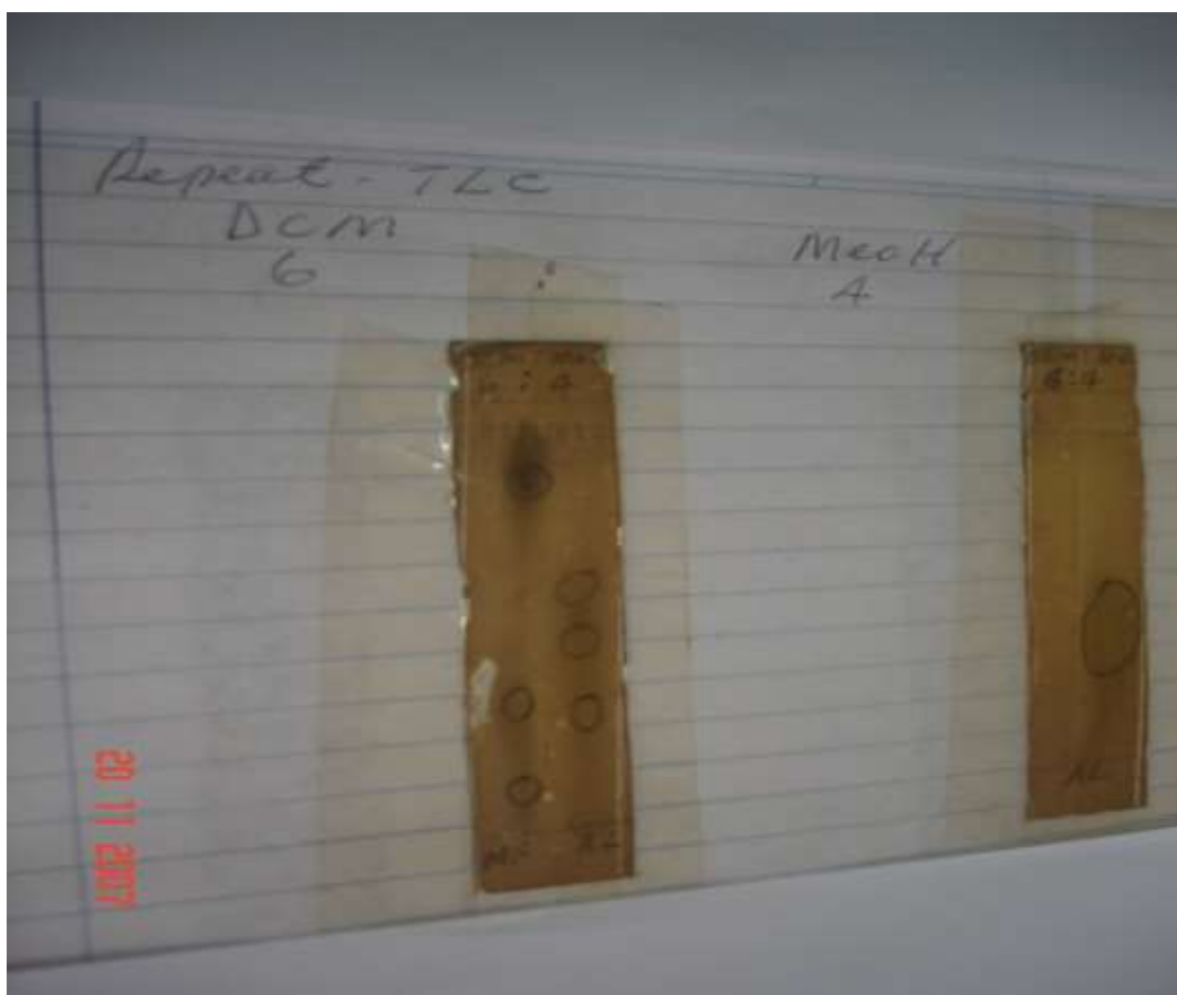
Figure 4.8: TLC profile of Chenopodium ambrosoides Methanol (fruit) Crude Extract using DCM: MeOH (3: 2) solvent system
